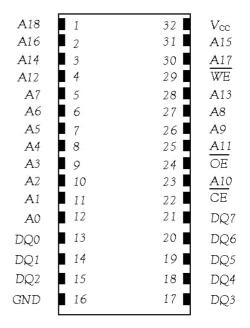
32-Pin Encapsulated Package 740-Mil Extended
